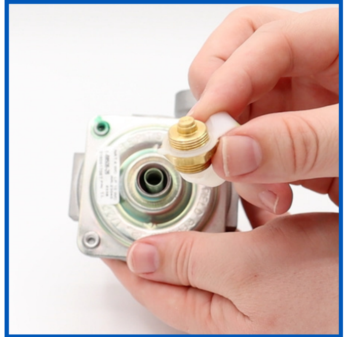
Remove the cap from the insert. Flip the insert over and replace the cap on the flip side.
